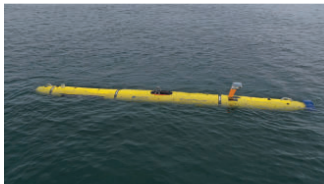
The General Dynamics Knifefish medium-class mine countermeasure UUV is designed for deployment off the Littoral Combat Ship (LCS) for detecting, classifying and identifying buried mines and mines in high-clutter environments.
