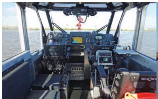
Metal Shark's Sharktech 29 Defiant boat has been converted to unmanned surface vessel ) via the use of Sea Machines' SM300 autonomous command and remote-helm control technology.
