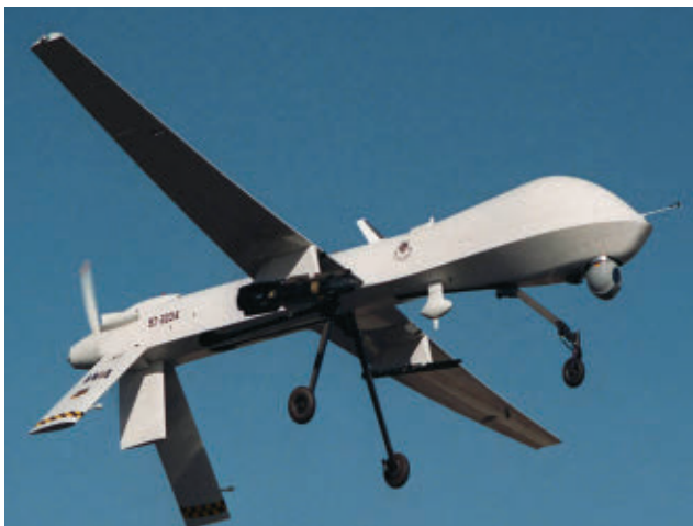
The MQ-1B Predator is an armed, multi-mission, medium-altitude, long-endurance remotely piloted aircraft that is employed primarily as an intelligence-collection asset and secondarily against dynamic execution targets.
