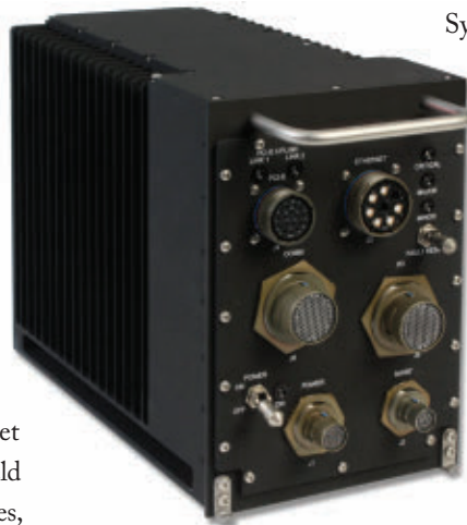
▲ This 1/2 ATR enclosure from Pixus typically uses OpenVPX in three to six slots, offers conduction cooling, with options for sealed versions with heat exchangers for high-power systems.
