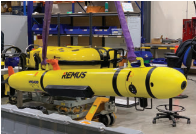
The Remote Environmental Monitoring UnitS (REMUS) 100 is a compact, light-weight, autonomous underwater vehicle designed for operation in coastal environments as deep as 100 meters.
